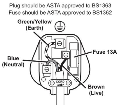
Ensure that the outer sheath of the cable is firmly held by the cord grip
