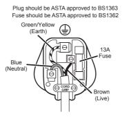
Ensure that the outer sheath of the cable is firmly held by the cord grip
