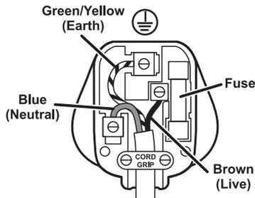
Ensure that the outer sheath of the cable
