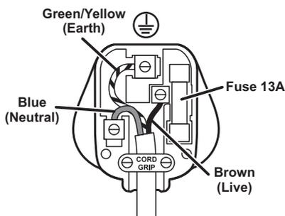
Ensure that the outer sheath of the cable is firmly held by the cord grip
