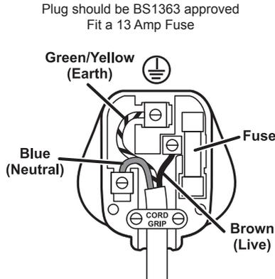
Ensure that the outer sheath of the cable is firmly held by the clamp
