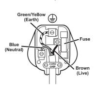
Ensure that the outer sheath of the cable is firmly held by the clamp
