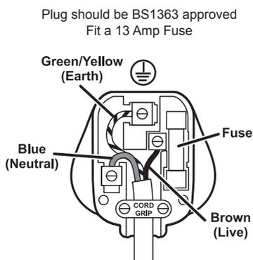
Ensure that the outer sheath of the cable is firmly held by the clamp
