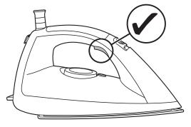
Press the steam trigger when steam is needed.
