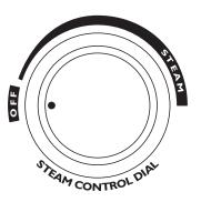
Turn the steam control anticlockwise to the OFF position. If you don't do this, water can drip from the soleplate during ironing.
