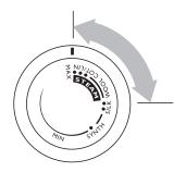
Turn the temperature control to the desired heat setting. For steam ironing, this MUST be between ●● and MAX otherwise water will drip from the soleplate during ironing.
