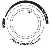
Turn the steam control to select the desired amount of steam. Turn it anticlockwise to decrease and clockwise to increase the amount of steam.
