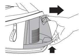
Press the red tab under the tank and slide the tank out. Fill it with water up to the MAX mark.
