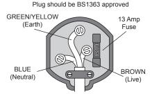
Ensure that the outer sheath of the cable is firmly held by the clamp
