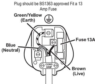
Ensure that the outer sheath of the cable is firmly held by the clamp
